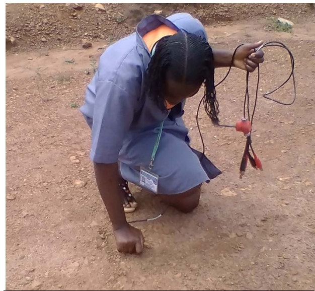
Fig.4: (i & ii): Setting up of the Seismic Traverse Line and inserting geophones into the earth
